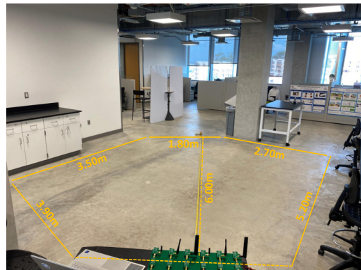
Figure 19: The area of interest for target location. The maximum distance from the radar is around 6 meters.
