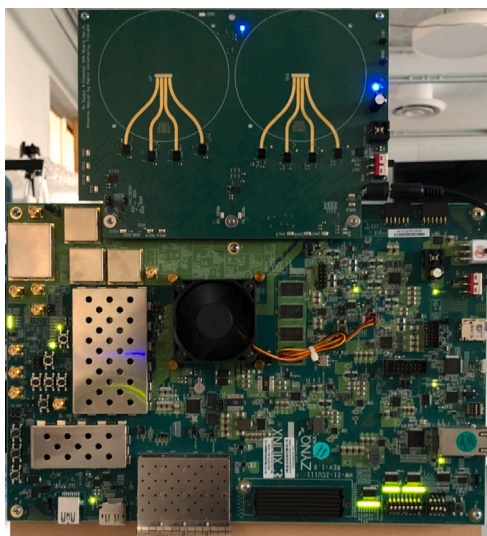
Fig. 2. The Pi-Radio v1 SDR being tested at NYU. The bottom board is the Xilinx RFSoc-based ZCU111 evaluation board; the board at the top is the Pi-Radio transceiver board. The RF shield has been removed to show the transceiver board clearly.
