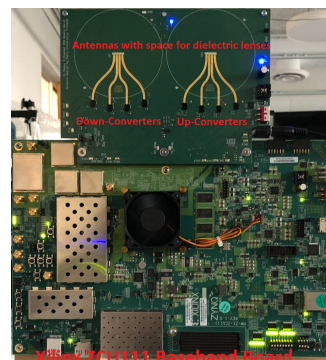
Figure 1: The Pi-Radio v1 SDR being tested at NYU. The bottom board is the Xilinx RFSoc-based ZCU111 evaluation board; the board at the top is the Pi-Radio transceiver board.
